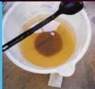
Floc formation after chemical addition
